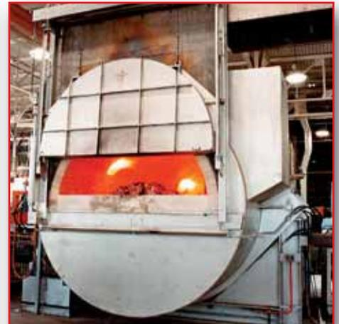
Barrel Melting Furnace
